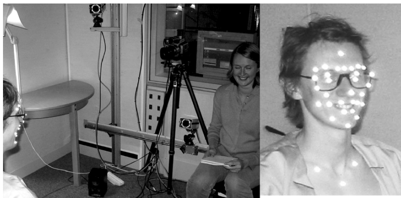
Figure 3. Data collection set-up with video and IR-cameras, microphone and a screen for prompts (left), and test subject with the IR-reflecting markers glued to the face (right).
